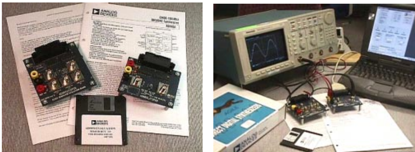
Figure 12-1. Typical Evaluation Kits for DDS Products
